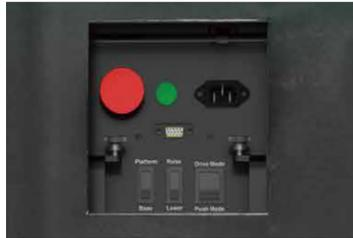
A lower operation panel is designed to enable the operations such as operation platform lifting, brake release, etc. to be performed outside the vehicle so as to facilitate vehicle maintenance.
