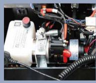
Integrated hydraulic unit, compact structu less space
