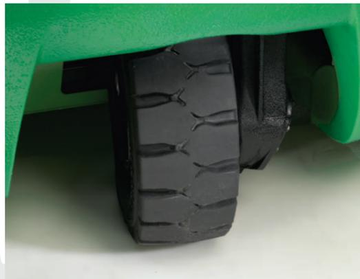
The 180° rotation of the rear single wheel, combined with the machine's compact size, allow excellent manoeuvrability even in tight spaces and narrow storage aisles.
