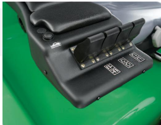
The proportional electronic controls integrated in the new (optional) armrest enable the operator to manage all the hydraulic functions by simply moving the Mini-Joystick or Fingertips levers.
