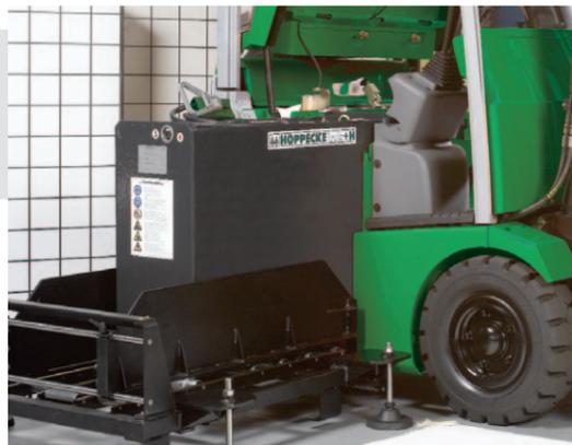
The optional lateral battery extraction allows battery change times to be minimised, optimising the truck's productivity.
